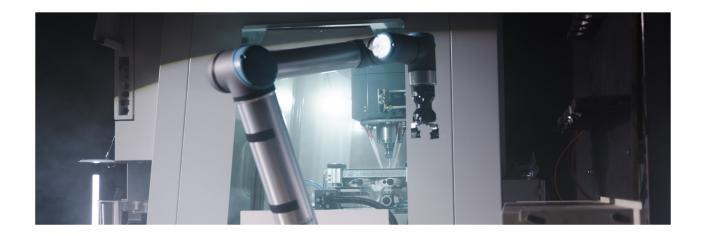
Coordination of machine and cobot: Insert parts from a location or a grid into a machine, activate the machine, and remove the part from the machine onto another location or grid. The extended range from the XtendR allows the cobot to reach new heights of the machine, feeder and shelf.
