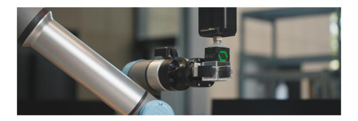
Transfer parts from a static location or a grid to another location or grid. The extended reach from XtendR allows the cobot to pick & place from various heights and locations.
