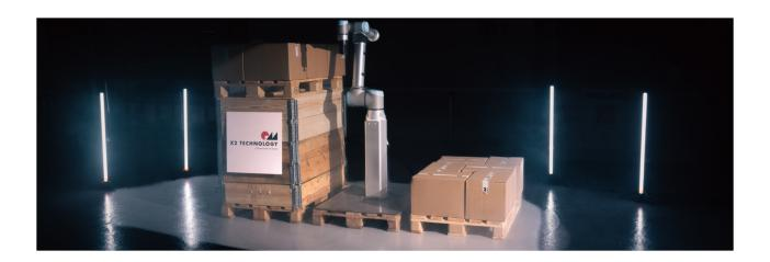
Pick parts from a static location, for example a conveyor or a grid and stack/pack them in a predefined pattern at a target location such as pallet, grid or box. The extended reach from XtendR allows the cobot to palletize in several layers to optimize the packaging line.
